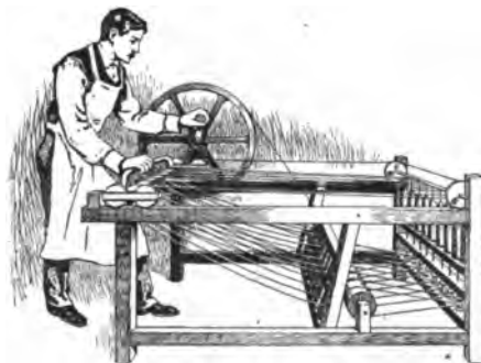
FIG. 154. THE FIRST SPINNING JENNY
